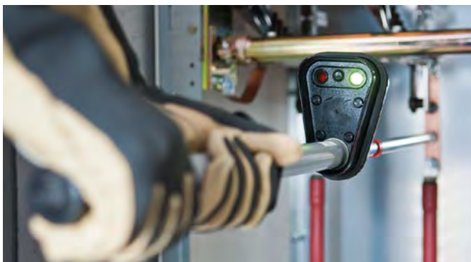
PHE voltage detector with visual indication
