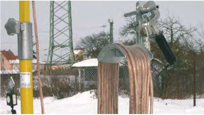
Earthing spike with coiled earthing cable.
