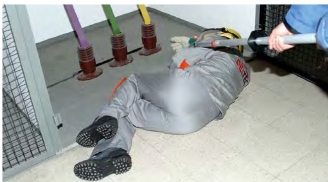
Insulated RST rescue rod used to rescue a victim of electrical shock from the live working zone
