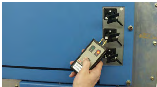
Self-test of a DEHNcap/A voltage indicator
