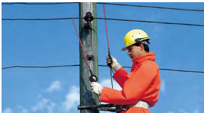
Two-pole SPN voltage detector used with extension prods for overhead lines
