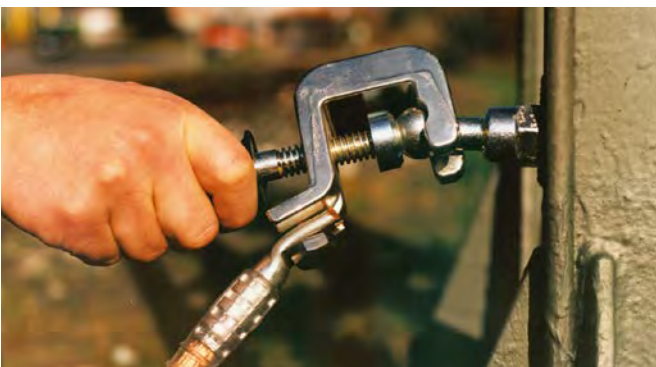
Universal earth clamp with handle connected to a fixed ball point
